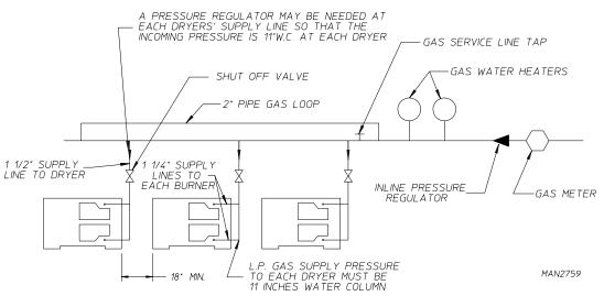
Consistent gas pressure is essential at <u>ALL</u> gas connections. It is recommended that a 2-inch pipe gas loop be installed in the supply line serving a bank of dryers. An in-line pressure regulator **must be** installed in the gas supply line (header) if the (natural) gas pressure exceeds 12.0 inches of water column pressure.
