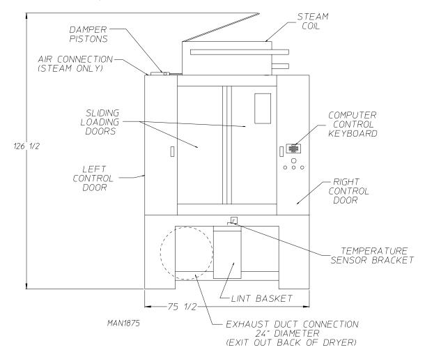
c. No air regulation is provided with a standard AD-310 dryer. External regulation/filtration of 80 psi **must be** provided. It is suggested that a regulator/filter gauge arrangement be added to the compressed air line just before the dryer connection. This is necessary to insure that correct and clean air pressure is achieved. The F/L/R/G is provided on dryers with the *optional* automatic door or the *optional* sprinkler circuit.
