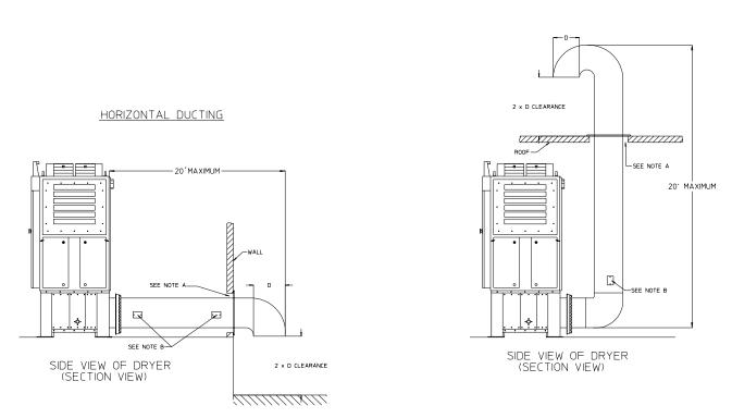
NOTE: "A"- OPENING MUST BE TWO (2) INCHES LARGER THAN DUCT (ALL THE WAY AROUND). THE DUCT MUST BE CENTERED WITHIN THIS OPENING.
