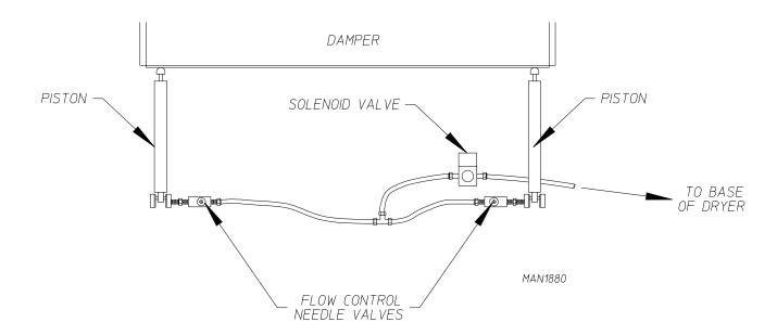
**NOTE:** TURNING KNOB ON FLOW CONTROL CLOCKWISE WILL RESTRICT AIR FLOW. TURNING KNOB COUNTERCLOCKWISE WILL ALLOW HIGHER AIR FLOW.
