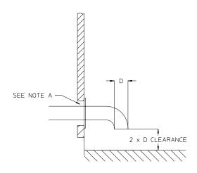
NOTE "A": OPENING MUST BE TWO (2) INCHES LARGER THAN DUCT (ALL THE WAY AROUND). THE DUCT MUST BE CENTERED WITHIN THIS OPENING.
